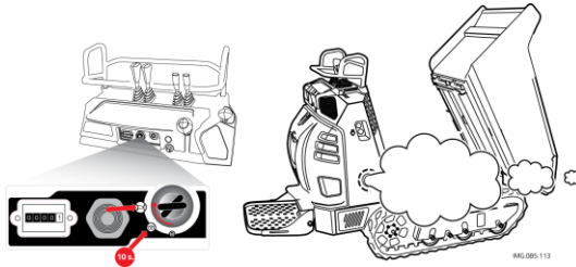
fig. 31– Verification of plugs preheating system
